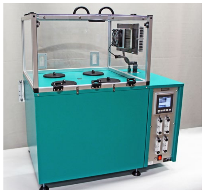
Temperature cycling oven EB 21LTHTP for relaxation tests with 4 cells with individual temperature control and cycling between RT to elevated temperature.
