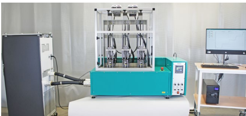
The EB 32.01 liquid circulator for cooling to the left of the automatic relaxation and creep tester EB 32, which can cycle between -40 °C and +200 °C, with the same temperature in all test stations.
