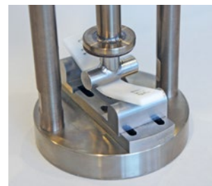
EB 02.29 Fixture for flexural creep by 3-point loading, according to ISO 899-2.
