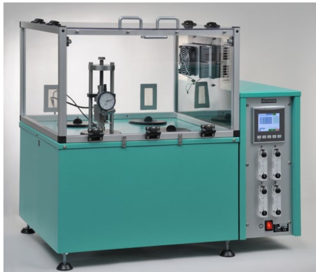
Cell oven, EB 21. For relaxation tests with 4 cells with individual temperatures.
