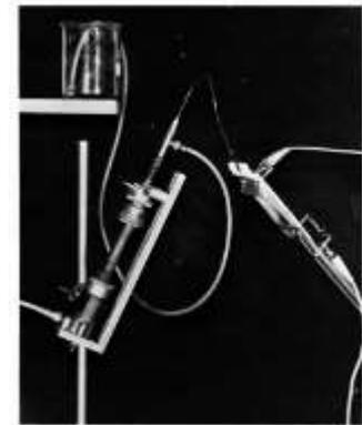
Top and bottom electrodes material: Stainless steel
