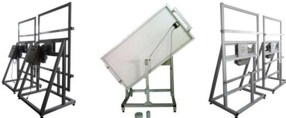
**Ud Torque test: (IEC 61215:2005, IEC 61646:2008)**
