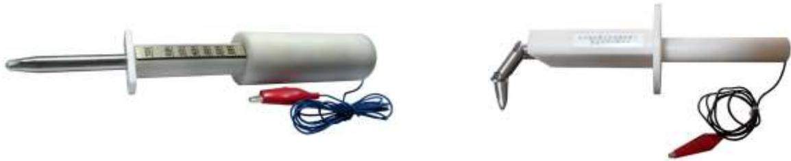
This probe may be used to verify the protection of persons against access to hazardous parts, and to verify the mechanical strength of openings in the enclosure or internal barriers.
