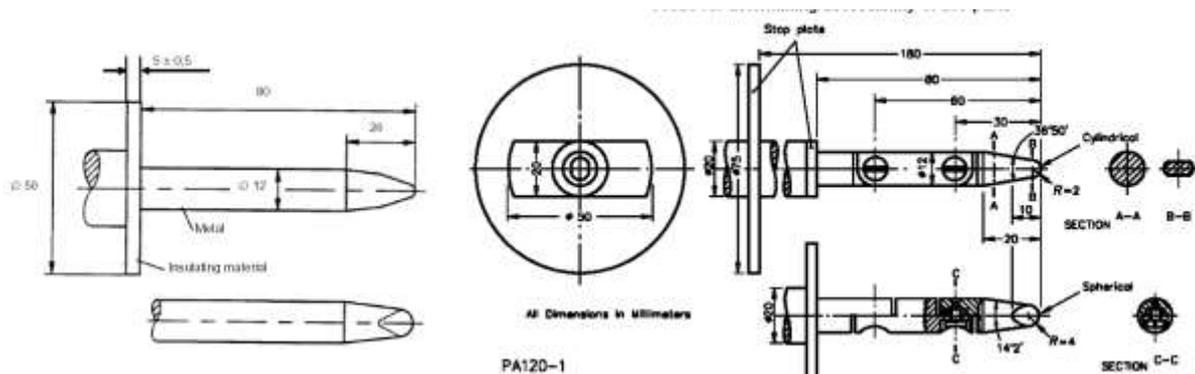
Application in VDE 0126-5 and VDE 0126-3, junction box and connector test conditions are as follows:
