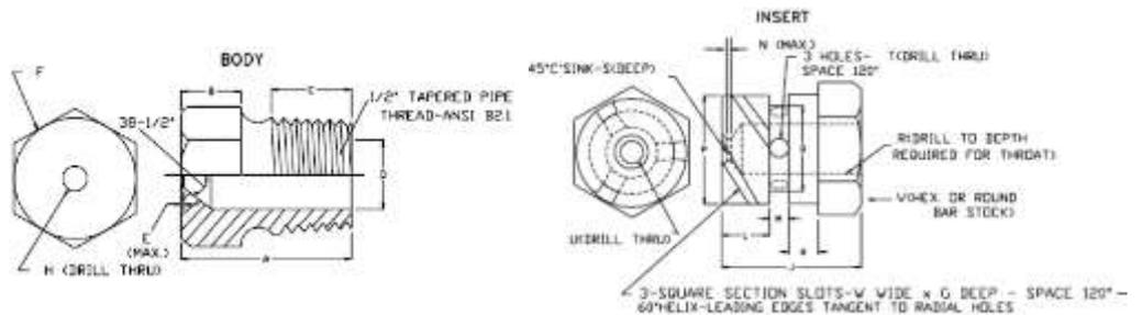
Test spray heads material: Molded nylon rain (see UL 1703)
