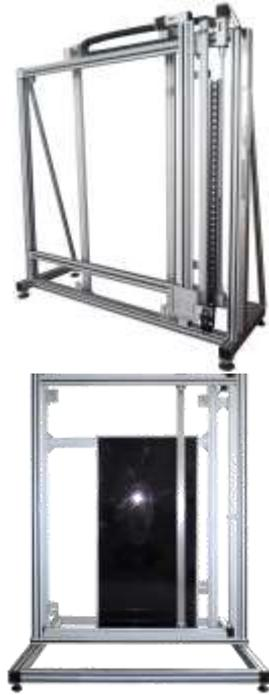
**Shading plate for hot-spot endurance test:**
