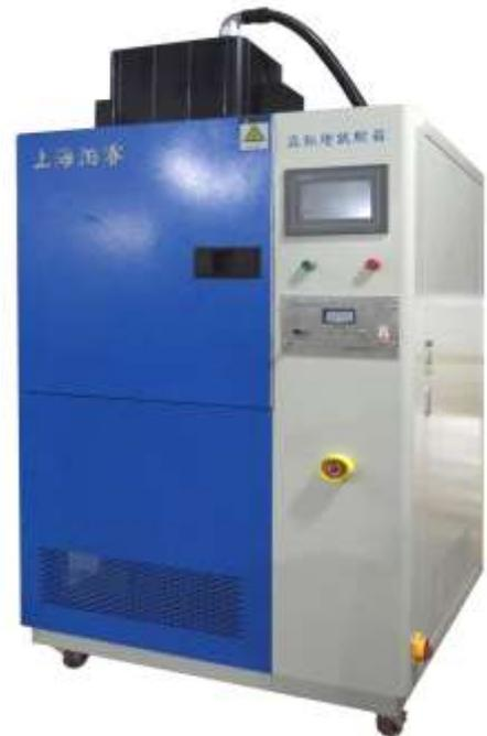
① DayLight filter: for junction box and connector test, spectral distribution conform to ASTM G155 and ISO 4892-2 requirements.
