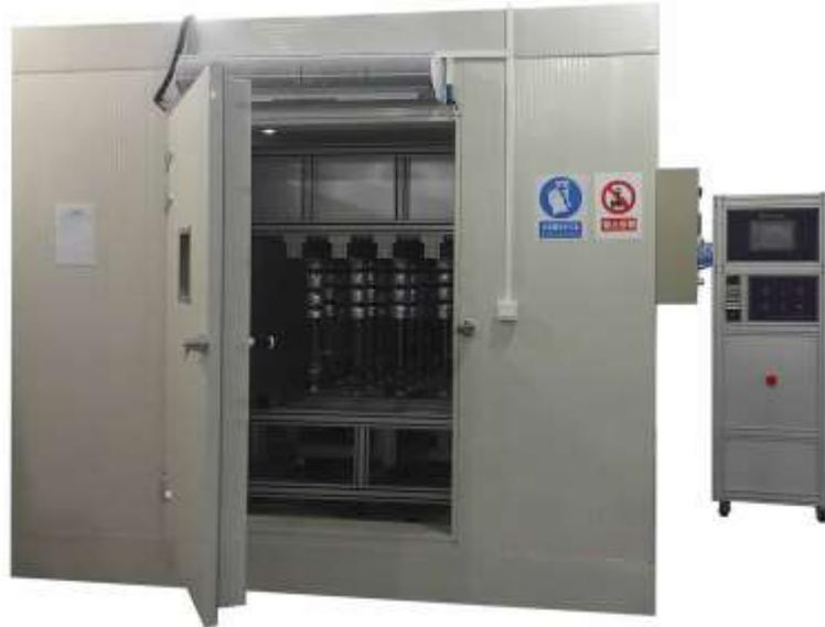
Extremely cold environment dynamic and static load test
