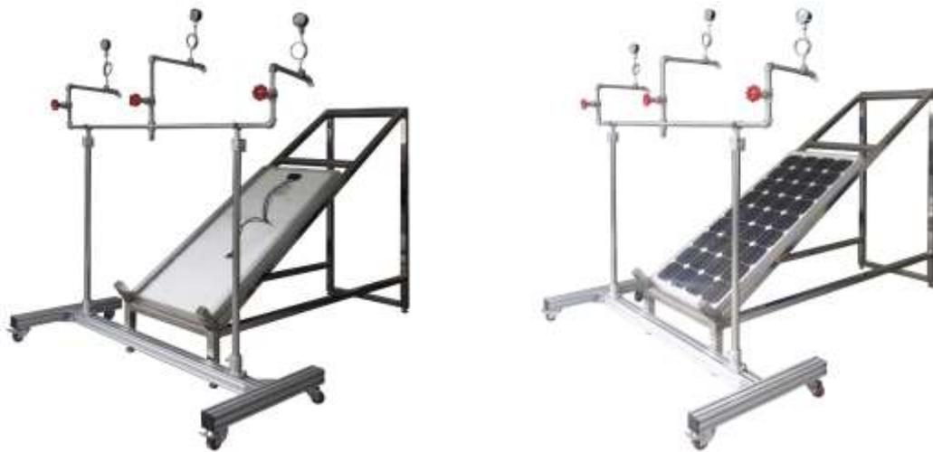
Module mounting angle 35° with the horizontal plane.
