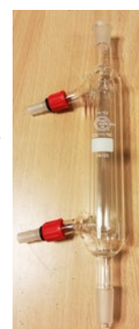
Water cooled condenser EB 11.04
