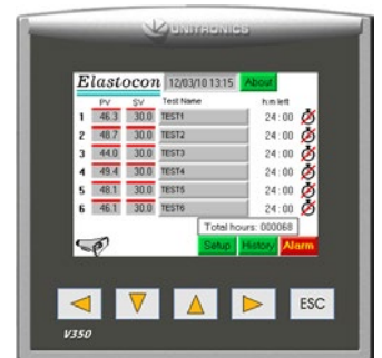
All ageing ovens are controlled from a colour touch screen.
