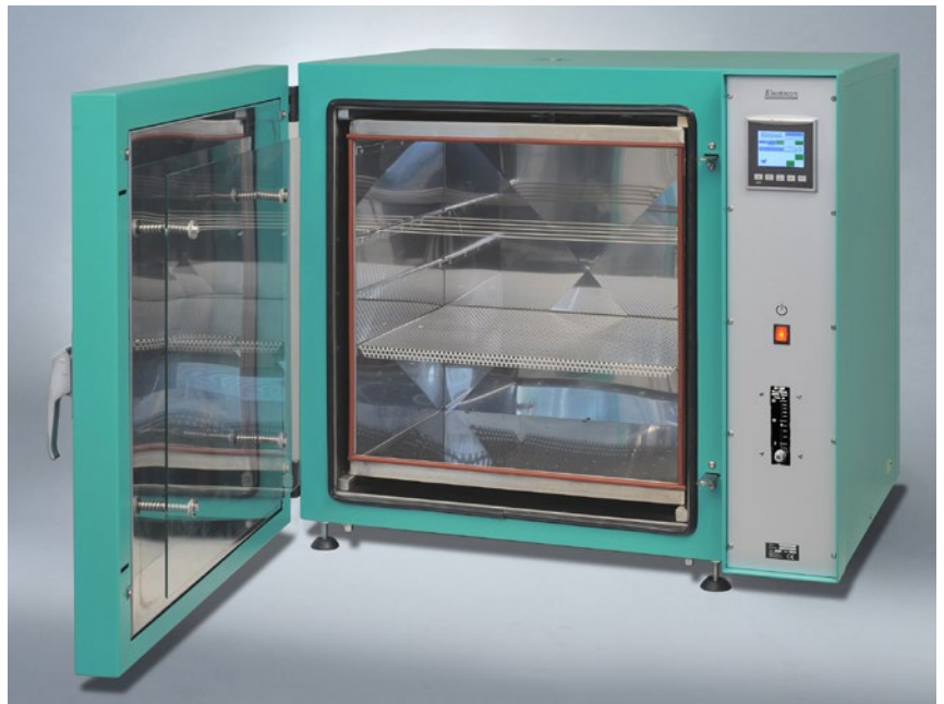
Cabinet oven EB 04-II with air supply that requires external air and a flow meter that can be set between 3 to 20 changes per hour.
