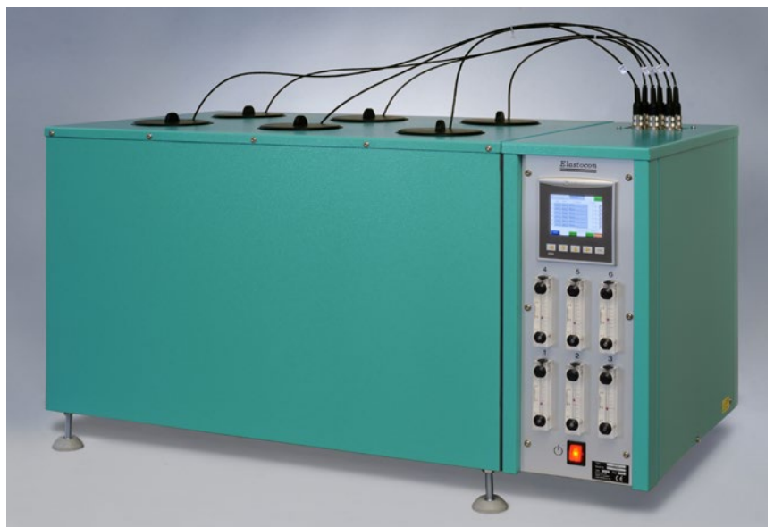
Cell oven EB 20 equipped with 6 cells, each with individual temperatures, and flow meters that can be set between 3 to 20 changes per hour.
