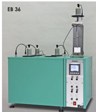
The EB 36 cell oven has a stirrer (detail to the right), that stirs the air in the cells with about 60 rpm and meets the standard AS/NZS 1660.2.3:1998.
