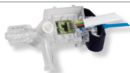
Laser soldering of wires on a ceramic substrate of a medical pressure sensor
